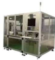
FC CSP Bump Inspection
